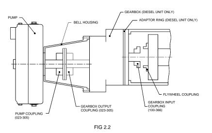
Fig 2.2 Pump Installation – Prime Mover/Gearbox/Pump Coupling Arrangements
