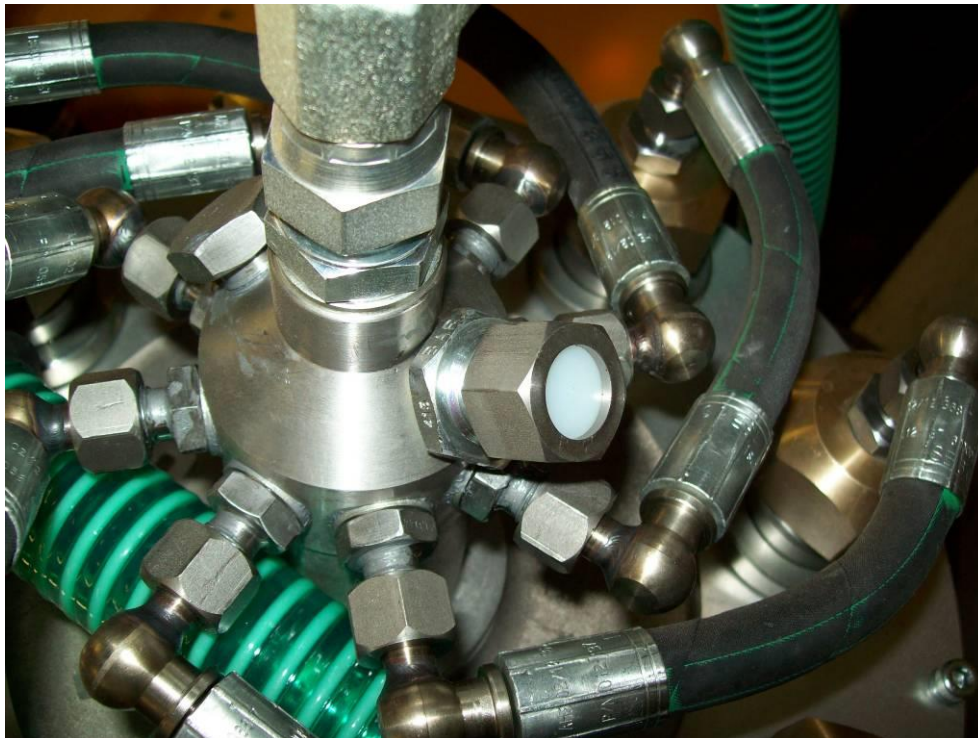
(Burst disc holder showing "White" burst disc)
