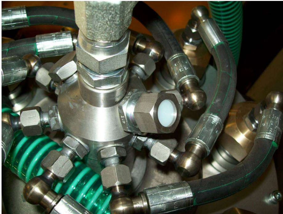
(Burst disc holder showing “White” burst disc)
